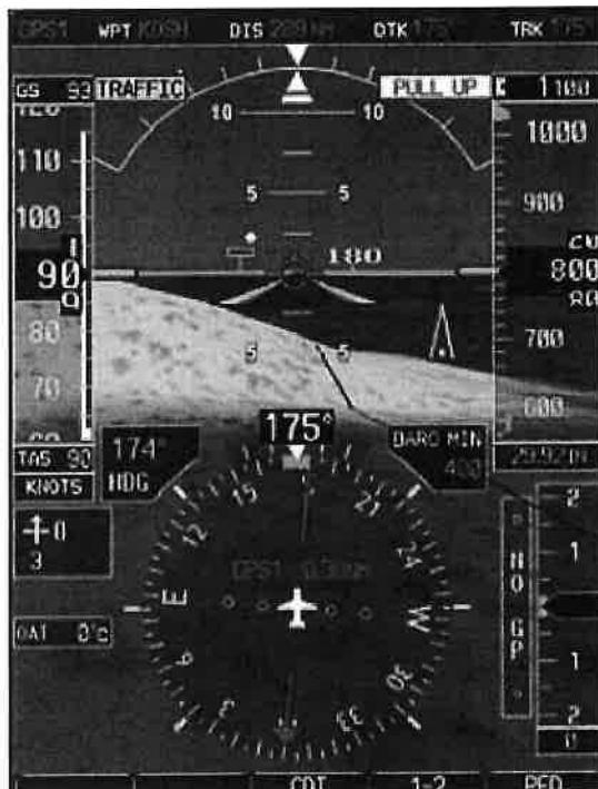
SVT provides additional features on the G500 primary flight display (PFD) which display the following information:
